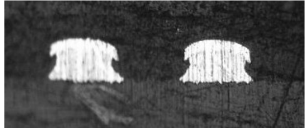
Figure 13: Microphotograph of sectioned differential traces.
